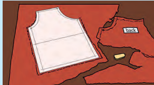
Figure 7.10: Uneven marking and cutting of fabric
